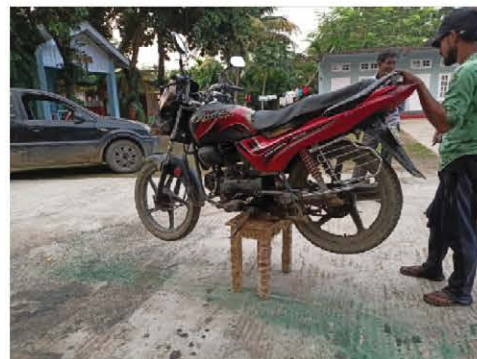
Demonstration of banana pseudo-stem composite stool strength
