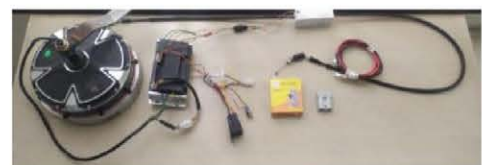
PHEV Kit and Motor controller with wiring connection
